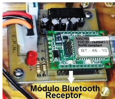
Figura 4.18 Módulo receptor Bluetooth
