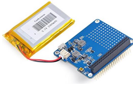
Figura 1.24. Raspi UPS HAT Board [49]
