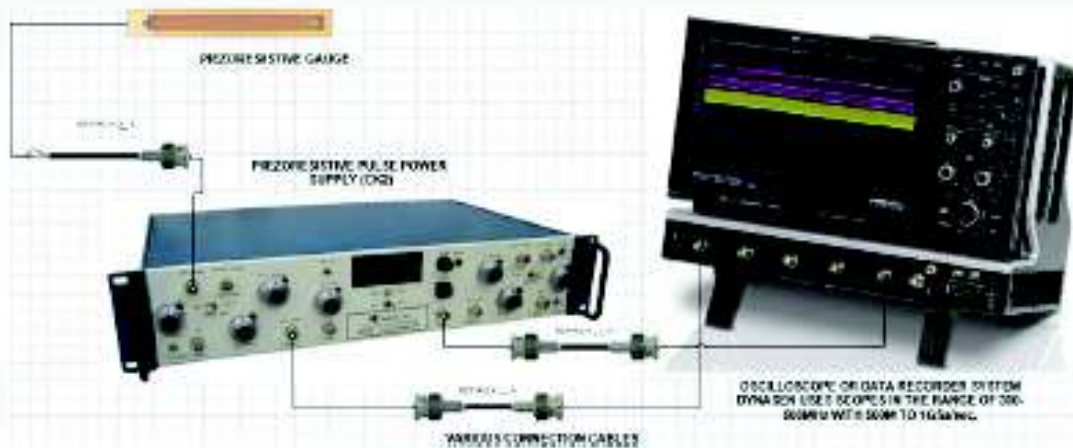
FIGURE 11. Generalized Component Set-up for Dynasen 50 ohm Piezoresistive Gauge Applications
