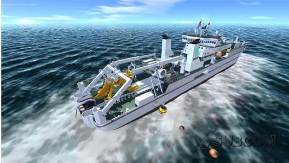
Cable Repair Ship is Positioned to Recover Buoy and First Cable End
