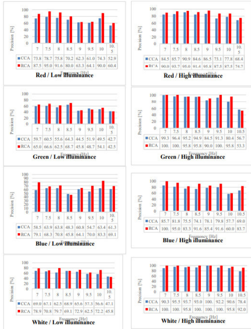
Fig. 4. Precision achieved with an LED of different colors, frequencies and illuminance
