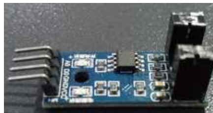
Figura 3.4 Sensor encoder FC-03.
