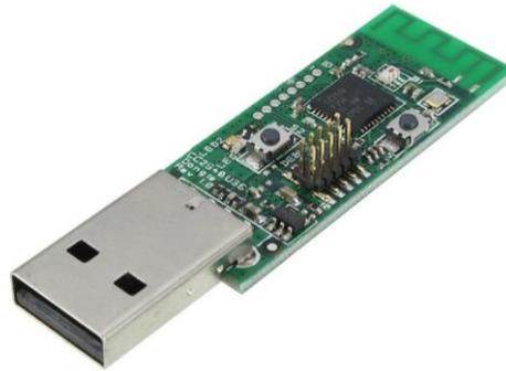
**Figura 2.9.** Sniffer Zigbee CC2531 USB Dongle [35].
