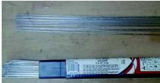
Figura 2.1. Varilla de aporte ER-2594 LINCOLN ELECTRIC.
