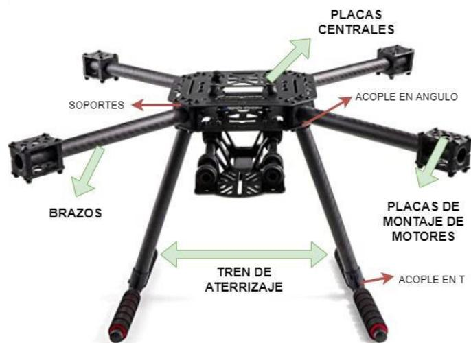
**Figura 3.1** Partes del dron comercial FPVKing 500-X4 [14]
