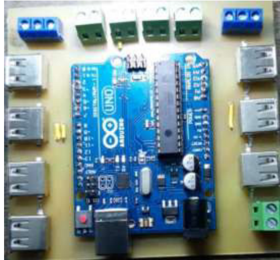
Figura 3-10 PCB de control
