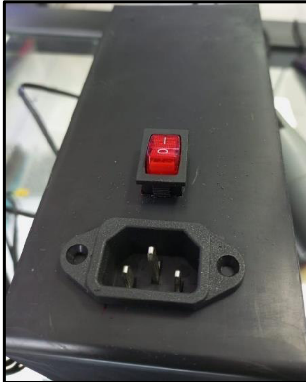
Figura 2.6 Interruptor general instalado
