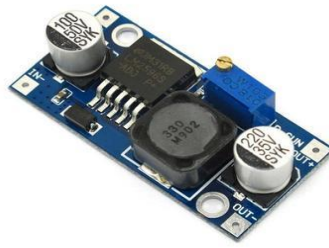
Figura 2.9. Reductora variable, de 12 a 5 [V] [27]
