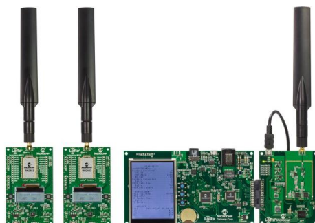
Figura 1.17 Gateway Microchip LoRa Technology Evaluation Kit – 800. Nodos RN2483 (izq.) y LoRaWAN Gateway Core + Radio Board (der.)[56].
