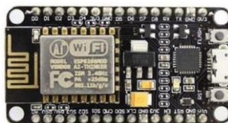
Figura 1.4 NodeMCU V2 ESP8266 [11]
