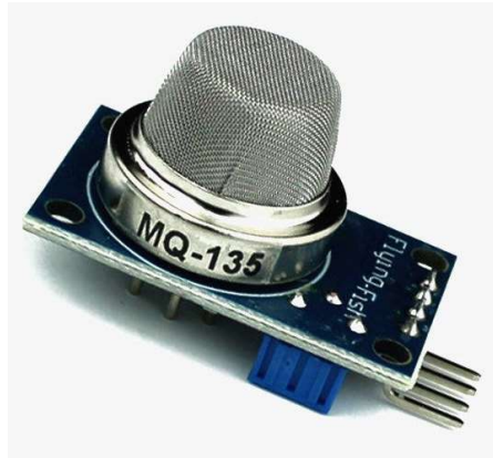
Figura 1.1 Sensor de gas MQ-135, [1].
