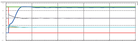
Fig. 16. Active power of the generators without UPFC
