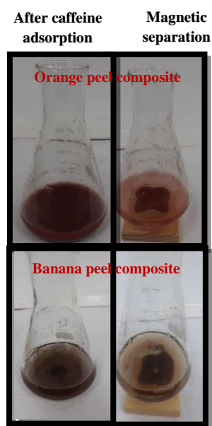
Figure 26. Photographs of the magnetic separation of the composites from the aqueous phase after caffeine adsorption.
