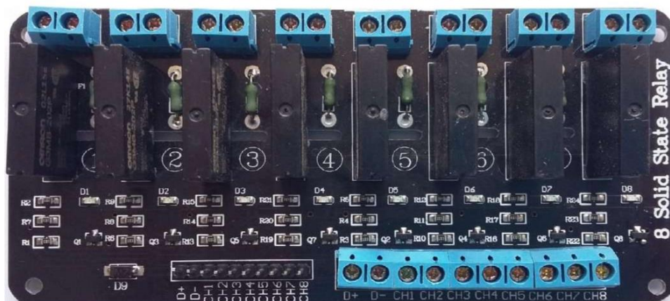
5V 2 A, 8 Channel SSR Solid State Relay Module Low Level Trigger
