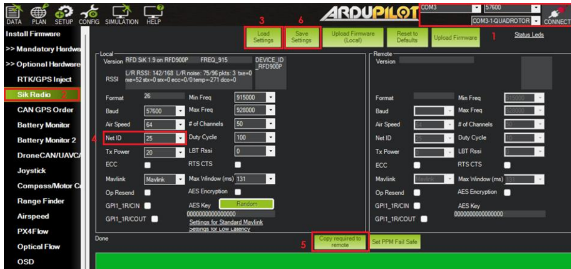
Figura 2.13. Mission Planner Sik Radio [Fuente propia]
