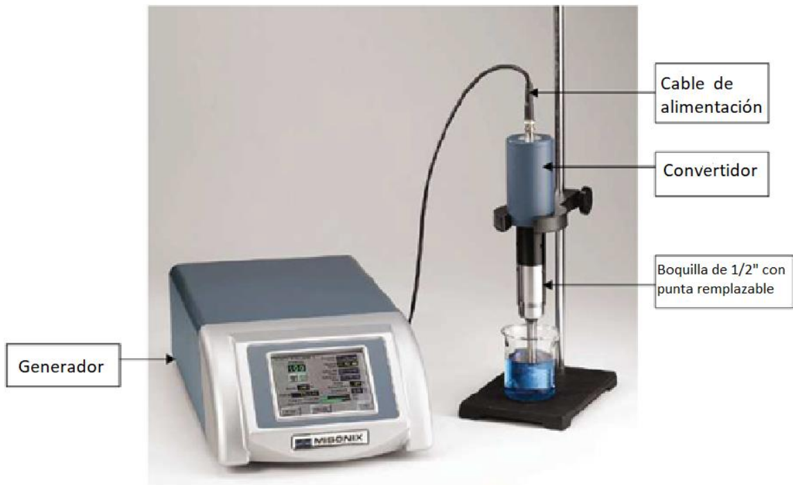
Figura 2. 5 Ultrasonido SONICATOR ULTRASONIC PROCESSOR S-4000 [74].
