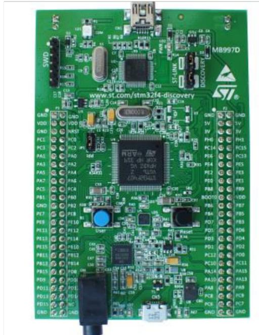
**Figura 1.20.** Tarjeta microcontroladora STM32F407G-DISCOVERY [12]
