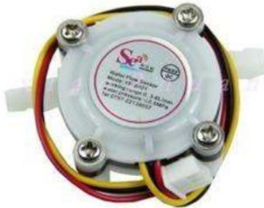
Figura 6. Sensor de flujo yf-s401 [17]
