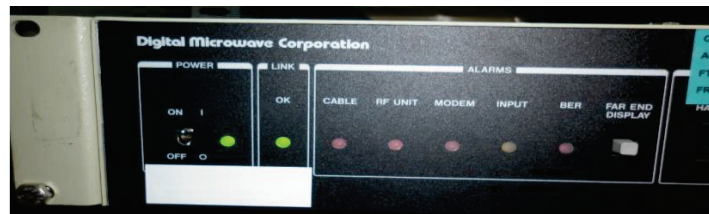
Figura 2.10 Modem de Radio DMC Classic II
