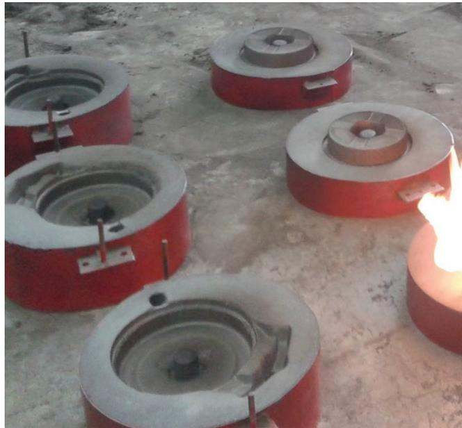
**Figura 4.2** Moldes Listos Para Colar
