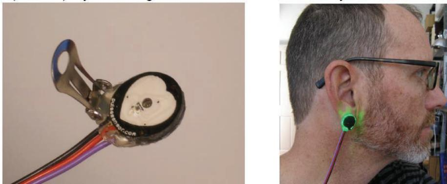
Take a good look at your work with a magnifying glass to be sure that you haven't made contact with any of the solder joints, then plug it in and test it. Hot glue is also great because it is easy to remove or re-work if you need to.
