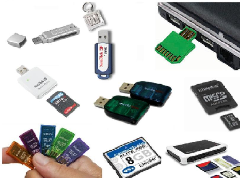
Figura 1.17 “Memorias Flash USB y Tarjetas Flash SD/MMC”
