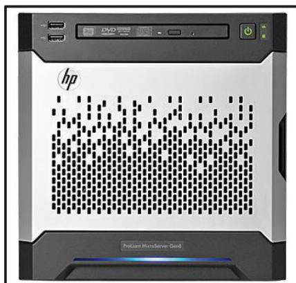
**Figura 4.11:** Servidor HP *ProLiant MicroServer Gen8*<sup>[77]</sup>
