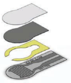
FSR 400 Short. Despiece tridimensional
