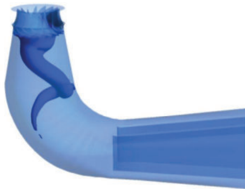
Figure 3.8: Vortex rope in draft tube (Zhang et al., 2012, p.7).
