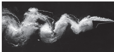
Figure 1.13: Example of cavitating vortices in the separated wake of a lifting flat plate with a flap. (E. Brennen, 1995, p.119)
