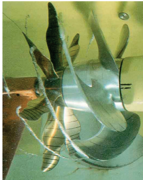
Figure 1.11: Tip vortex cavitation on a model propeller. (E. Brennen, 1995, p.118)
