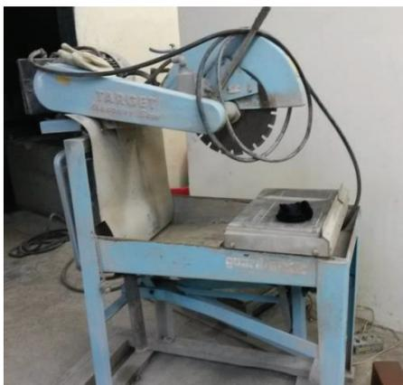
**Figura B. 1** Ingleteadora Target Mansonry Saw
