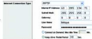
Figure 6-6: PPTP Connection Type
