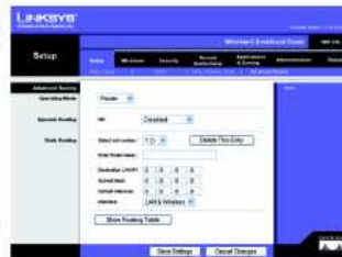
Figure 6-15: Setup Tab - Advanced Routing (Router)
