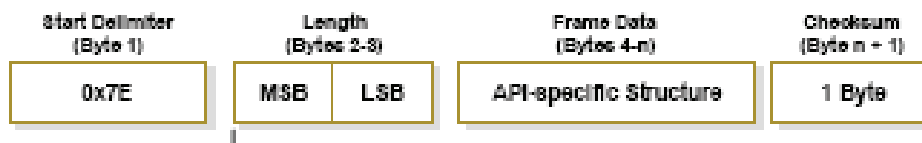
Figure 3-02. UART Data Frame Structure - with escape control characters:
