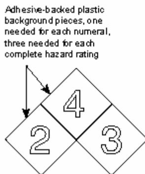
Figure 1 For use where specified color background is used with numerals of contrasting colors.
