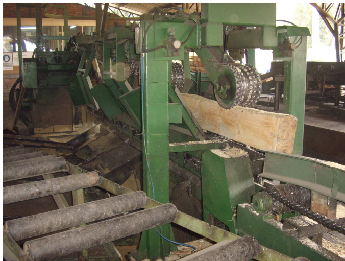
Figura 1.2.1 Corte principal - sierra KBO 40
