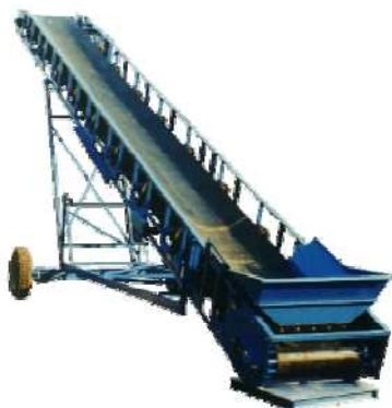
Figura 1.2. Cinta hueca (troughed belt conveyor)
