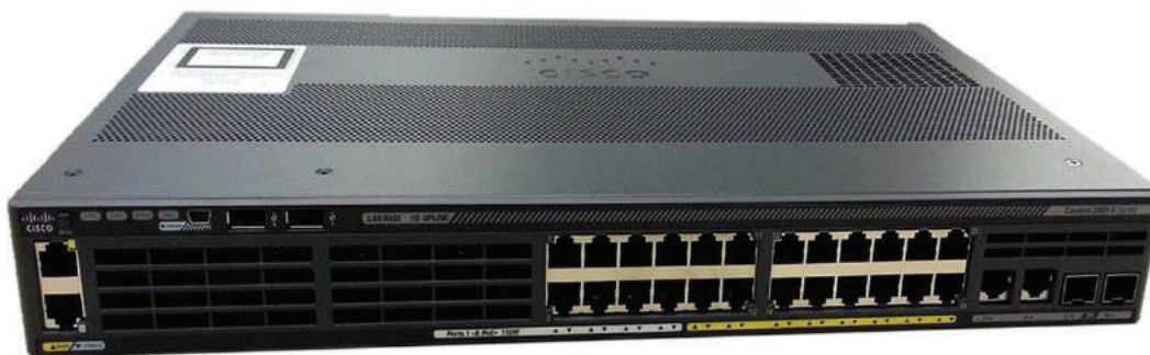
Figure 4. Fanless Quiet Cool 24-Port PoE Switch
