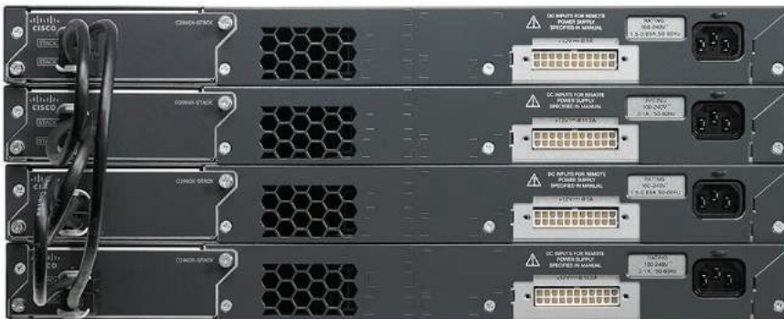
Figure 2. Cisco FlexStack-Plus Switch Stack
