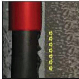
Fig. 1-B: As mud is smeared into the formation, filter cake builds up on the borehole wall.
