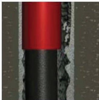
Fig. 1-A: Casing is forced against the bore wall as it advances into the borehole.
