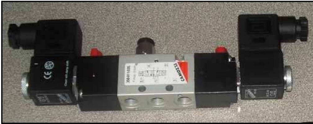
Fig. 2.17 Electroválvula biestable 5/2 CAMOZZI
