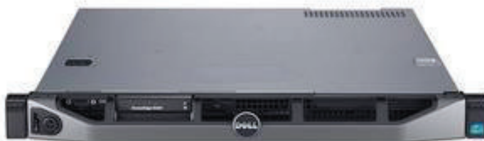
Figura 3.24 Servidor DELL PowerEdge R220 [59]
