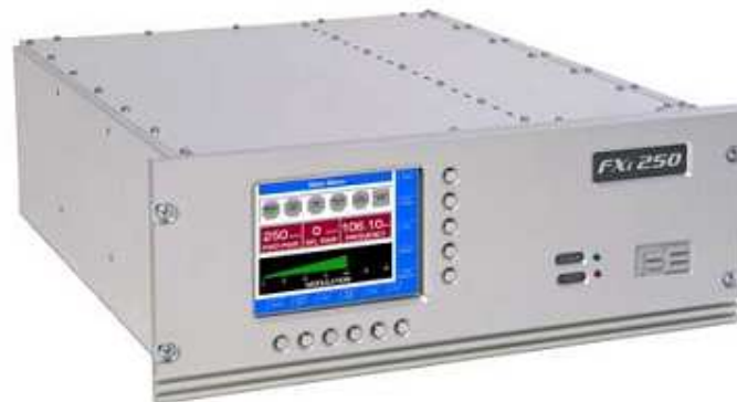
Figura 5.16 Excitador FXi 250 de Broadcast Electronics 48
