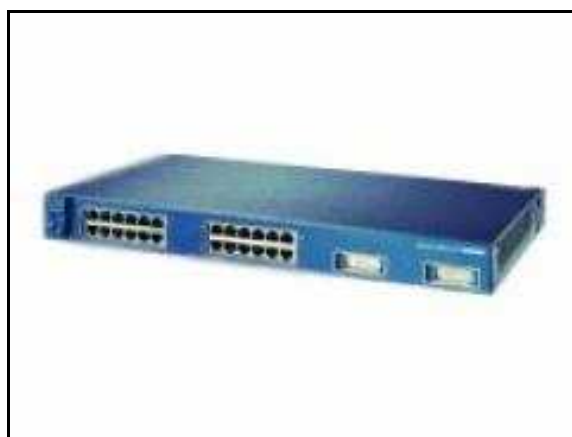
Figura 2.10 Switch Cisco Catalyst 3550
