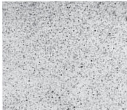
**Figura 6.33** – Microestructura de AA6061-TT<sup>37</sup>
