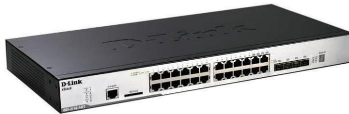
**Figura 44 - Switch Dlink DGS-3120-24TC-SI [49]**
