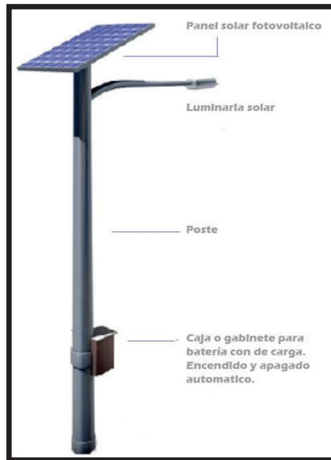
FIGURA 8-8. POSTE DE LUZ CON PANEL SOLAR
