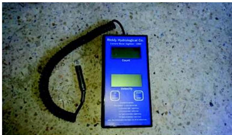
**Figura 26.** Contador de pulsos Rickly Hydrological Co.
