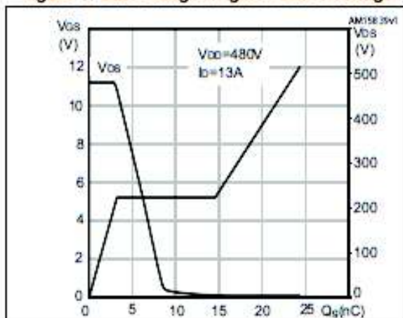
Figure 6. Gate charge vs gate-source voltage
