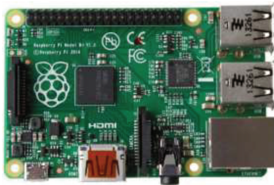
Fig. 4.6 Raspberry Pi Modelo B+
