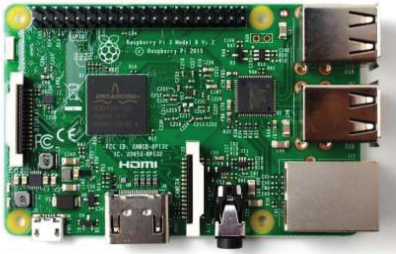
Fig. 4.8 Raspberry Pi 3 Modelo B
