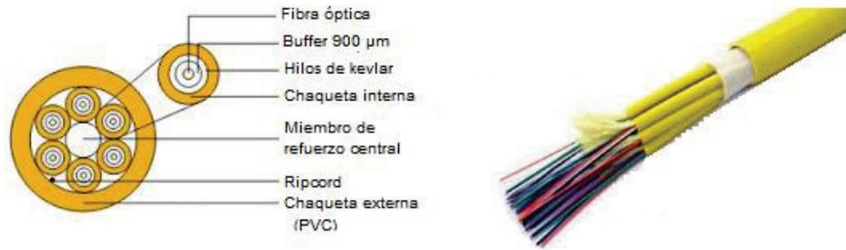
Figura 1.29 Cable *break out* <sup>[82]</sup> <sup>[83]</sup>
