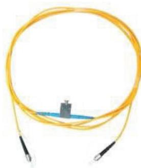
**Figura 2.18** Atenuador variable FIS F1-0031-LBR [109]
