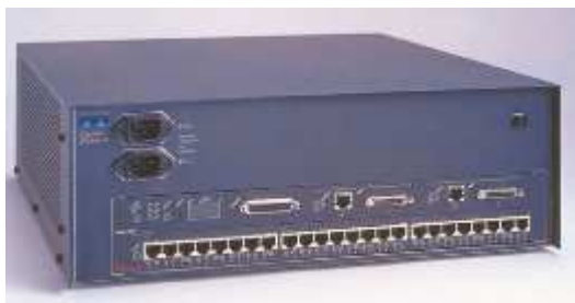
Fig. 25 – Switch de Capa 3 (Cisco Catalyst 2926G)
