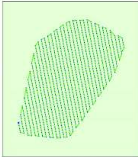
Figure 2: Top view of the initial image position. The green line follows the position of the images in time starting from the large blue dot.
